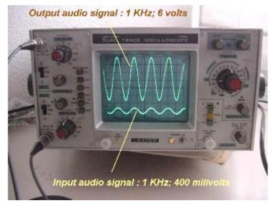
I found in my project that a signal of .4 volts, at 1 KHz, was amplified to an output of 6 volts. The audio signal amplified was an exact replica of the input, without any appreciable deformation. It is important not to introduce an excessive audio voltage to maintain the senoidal form of the wave.
