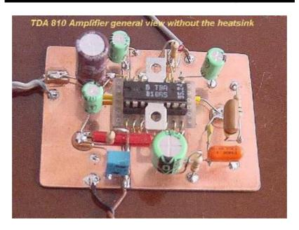
...built around the TBA 810 Integrated Circuit
