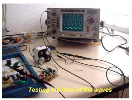
Heathkit Electronic Design Experimentor, which has frequencies from 200 Hz to 20 Khz. With a double-channel oscilloscope, you plug one of the channels to the input signal of the amplifier and the other channel to the output. Now you can compare the forms on the screen and see if the amplifier deforms the input signal.
